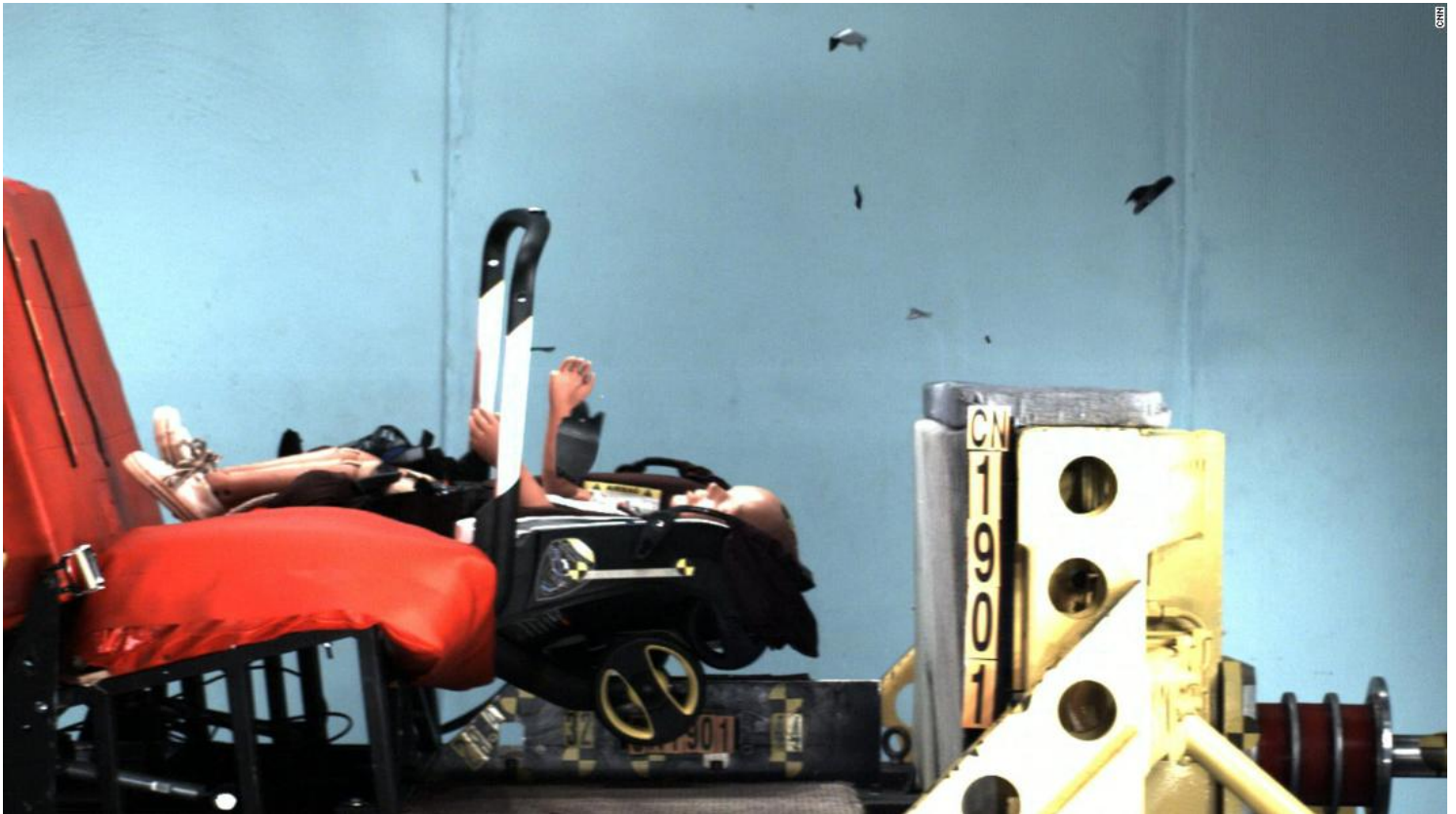
A car seat purchased on Amazon fractured in a 30 mph crash test, failing to meet federal standards
